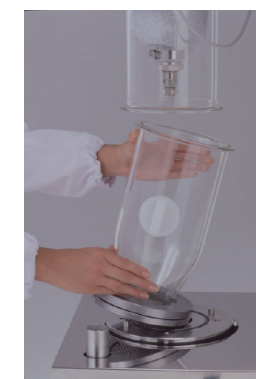
The upper and lower sections are divided to allow easy insertion of Sample compounds.
