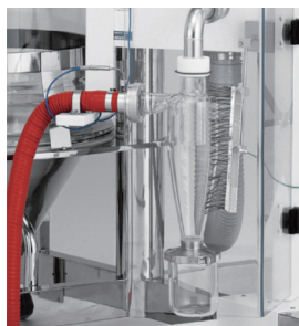
Cyclone separation section is equipped with burn prevention safety cover and the static removal brush.
